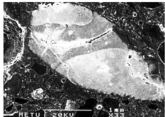
Fig. 3 SEM micrograph of cracked aggregate due to ASR in un-reinforced matrix
